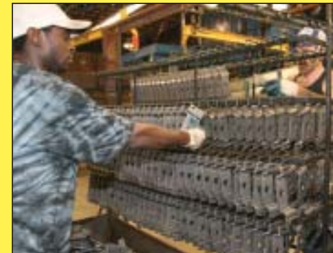
Fixtures are designed for "off-line" racking. Each part configuration has its own fixture to optimize handling, density and coating application.
